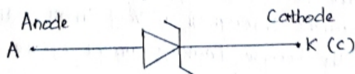
Fig. 1. Symbol of Zener diode
