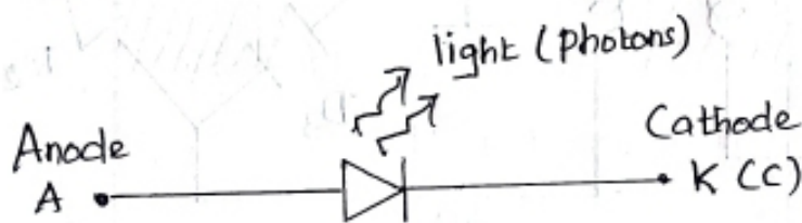
Fig. 1. LED and its symbol.
